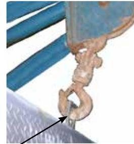
NOTE: Overall length of lifting chain and bracket (A) must be kept to a minimum to prevent interference between the lifting equipment and the building ceiling or door as the dock leveler is lowered into the pit.
